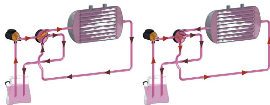
*The automatic flow inverter (patented) allows the attacking of the scales from both the inlets of the circuit and makes the machine particularly successful with almost totally obstructed pipes.*
